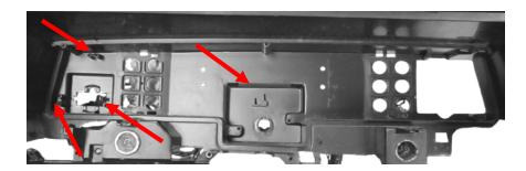
5. Route the provided Main Harness and the Buzzer (optional for audio feedback) through the back of the stock dash and connect to the back of the HDX system.
