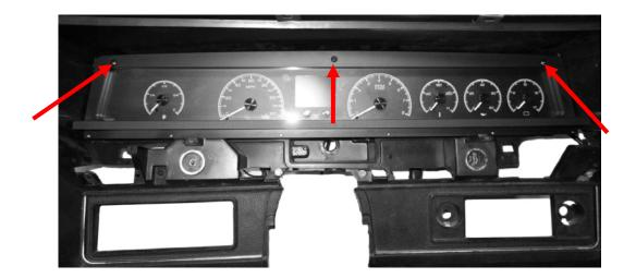
7. Re-install the lower gauge cover using the factory hardware and refer to the main manual for wiring instructions to complete the HDX installation.
