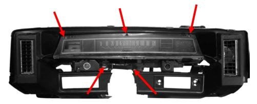
3. Remove the stock gauges, bulbs, and speedometer cable clamp. Set these items aside; they will not be reused.
