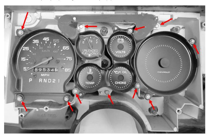
4. You should be left with a bare housing. Remove all light bulbs and electrical contacts, as they are not needed for the HDX system.
