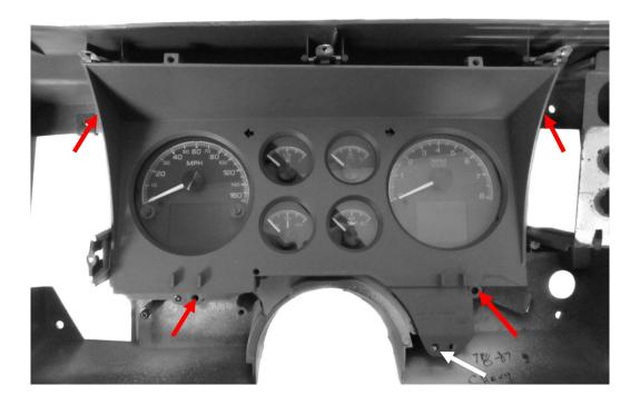
9. Reattach the bezel to the housing with the seven factory screws removed in Step One. Refer to the main manual for wiring instructions to complete the HDX installation.
