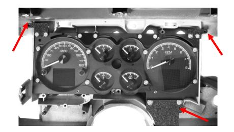
8. Separate the stock lens from the blackout plate; the original lens is not needed. Place the blackout plate over the Dakota Digital gauges while aligning the mounting holes. Attach the HDX system using the five factory screws. Place the included 1/8" white plastic spacer beneath the blackout plate at the lower-most mounting hole before installing the screw (white arrow).
