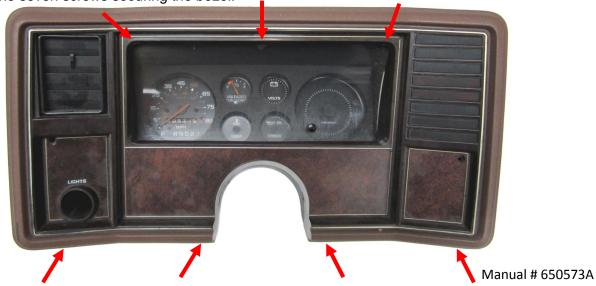
2. Remove the six screws securing the blackout plate and lens to expose the factory gauges. These screws will be reused.
