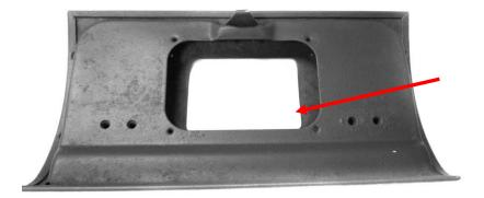
3. Carefully position the new clock from the backside to avoid scratching the chrome. With the four screws provided, secure the new clock to your original glove box.
