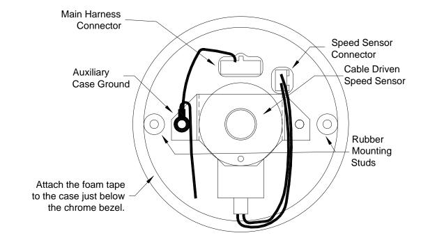
Mounting hardware and speed sensor connection for the clip-in system with an electric, transmission speed sensor.
