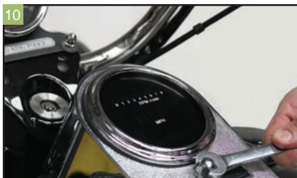
With the new gauge installed, place the instrument panel back onto the gas tank and secure it with the stock hardware.
