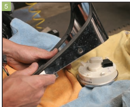
With the back clamp and wiring plug removed, remove the speedometer from the instrument panel.
