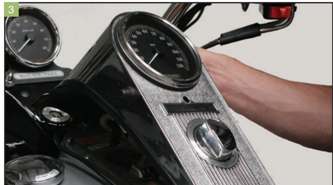
After removing the two dash fasteners, carefully lift the instrument panel off the gas tank.
