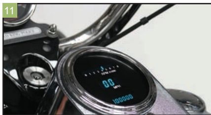
Reconnect the ground cable, and test the new digital gauge. The only thing left to do is remove the factory tach from the handlebar cover.
