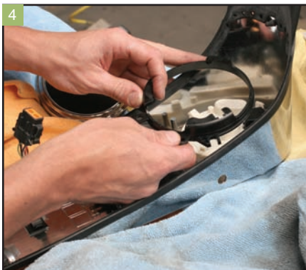
Next, remove the speedometer back clamp from the inside of the instrument panel.
