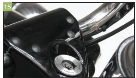
With the bolts removed, cover the holes with some plastic push-in clips from the automotive world.
