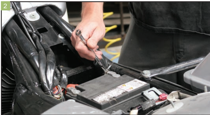
The first step is to remove the seat and disconnect the ground cable from the negative post on the battery.
