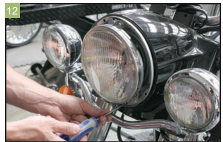
Remove the headlight trim ring and headlight, and then, disconnect the wiring for the tachometer.
