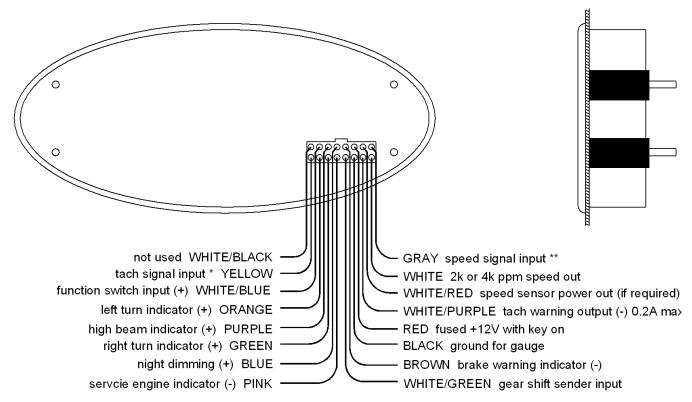
\* tach signal wire should be routed away from other signal wires.
