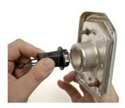
2. Remove the tail light housing hardware so the housing can be taken out of the car. Remove the housings from the vehicle carefully so the body gaskets are not damaged.
