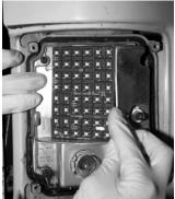
6. Before mounting the new LED assembly into the housing, plug the bulb base into the stock bulb socket and test the tail lights and flashers to make sure everything is working
