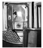
7. Make sure the tail light housings are clean and dry so the single use primer applicator can be used for both housings. Apply the primer to the outside edge of the housing where the tape will attach. AFTER THE PRIMER HAS BEEN APPLIED, LET THE HOUSING DRY FOR 5 MINUTES BEFORE GOING ON.
