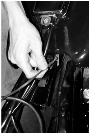
Route wires under tank
