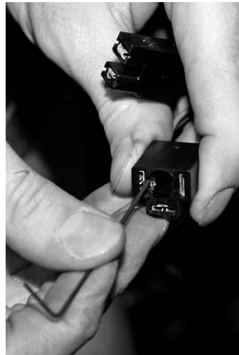
Push gently on the tab to release pin
