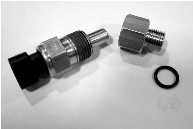
Oil temp sensor, adaptor bushing, and o-ring
