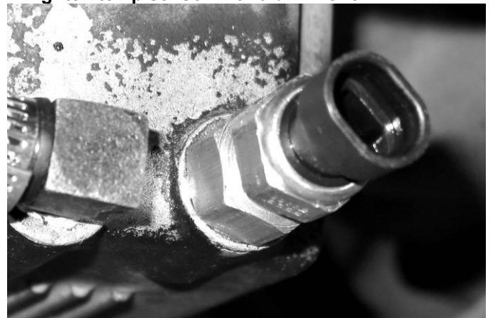
Temp sensor installed as drain plug EVO
