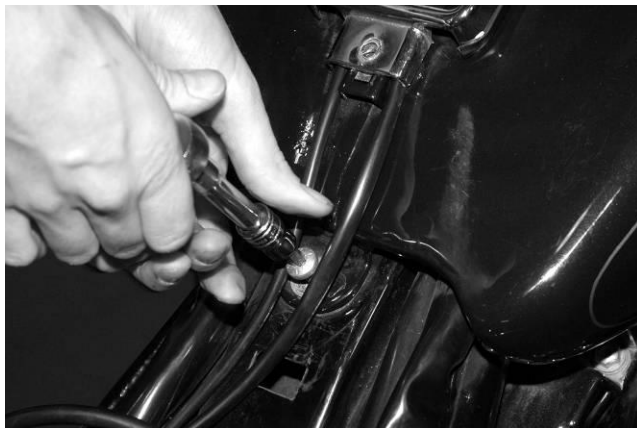
Remove rear tank bolt
