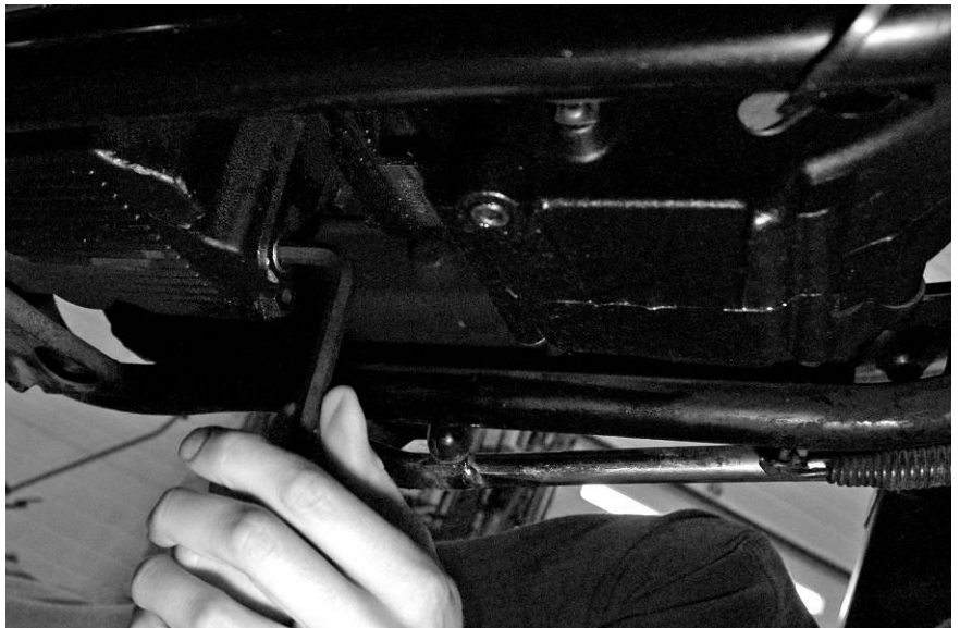
Remove 3/8" NPT allen plug
