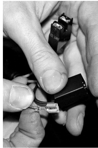
Remove the pin from the connector
