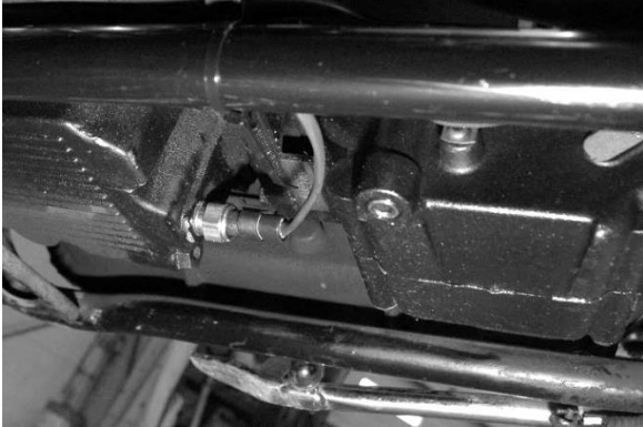
Installed oil temp sensor and harness plug
