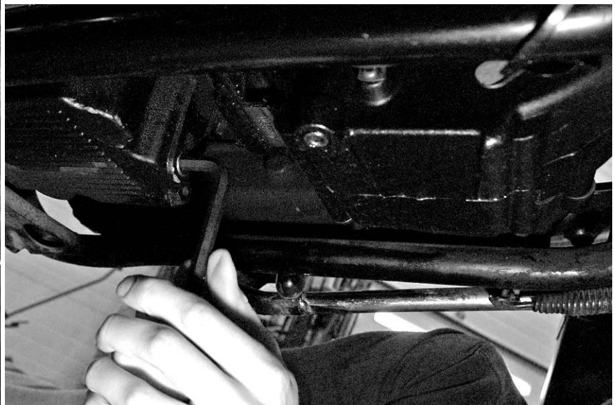
Remove 3/8" npt allen plug
