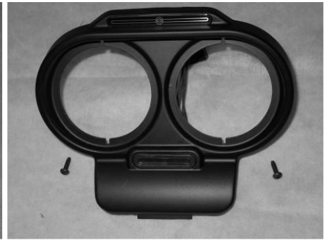
Gauges and gaskets removed
