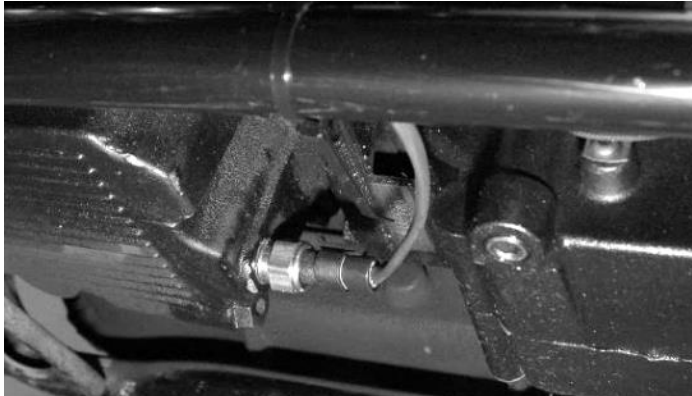
Installed oil temp sensor and harness plug
