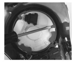
Ensure that the rubber gasket is still in the dash or remove from factory gauge and place back on dash.
