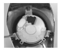
Remove the rubber gasket from the factory gauge
