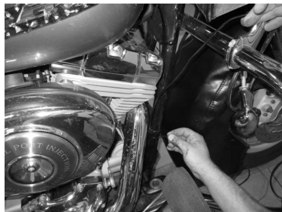
Tighten temp sensor with a 3/4" wrench
