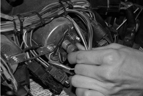
Remove speedo cable/unplug gauges
