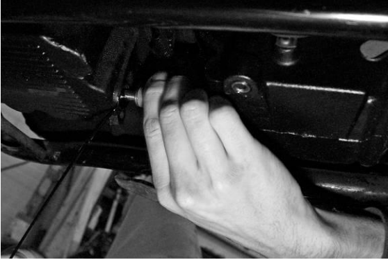
Thread sender into oil pan
