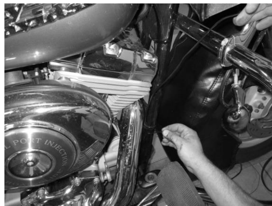
Tighten temp sensor with a 3/4" wrench
