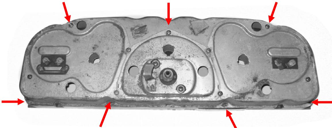
2. Remove the stock gauges, separator plate, and lens from the bezel. The only item to be reused is the original front bezel; the other pieces can be set aside. Cut the supplied foam tape into four pieces, so each is about two inches long. Cut them lengthwise to make eight thin strips; stick the foam strips on the angled part of the inside edge of the bezel. The lens will compress against any foam above the edge, which helps prevent lens rattles.
