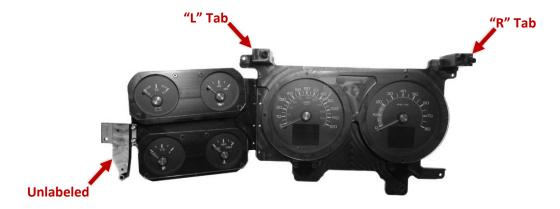
The remaining unlabeled tab goes on the bottom left side of the system, between the satellite gauges. Making sure the countersunk side of the tab is facing away from the rest of the unit, fasten this tab to the RTX system with the two included **6-20 x**  $\frac{3}{4}$ " flat head screws. This tab can be tightened until flush.
