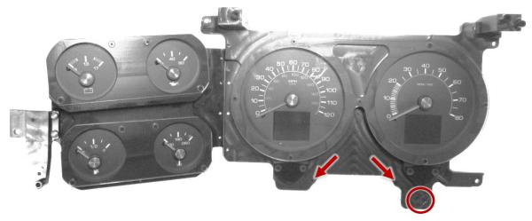
7. Install the stock bezel over the RTX gauge cluster using the stock screws removed in Step One. Tighten the locations shown below first to ensure proper fitment and alignment; if the holes are not aligned correctly, Step Three may need to be repeated.
