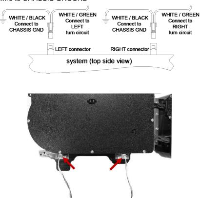
5. Connect the provided main harness and the buzzer (optional for audio feedback) to the back of the RTX system. Carefully route the main harness through the dash to the control box mounting location.
