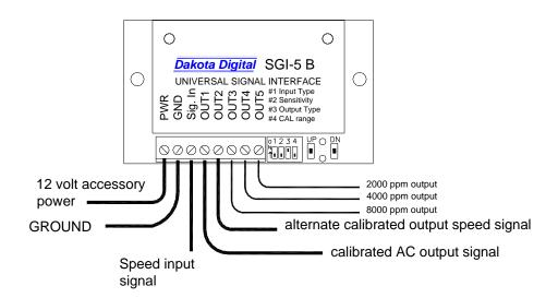
Recalibrate a low speed (8000ppm – 4000ppm) signal for an OEM or aftermarket speedometer or fuel injection computer.
