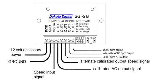
Convert a high-speed signal found on newer GM transmissions down to a low speed signal to run a speedometer, cruise control, or fuel injection computer.
