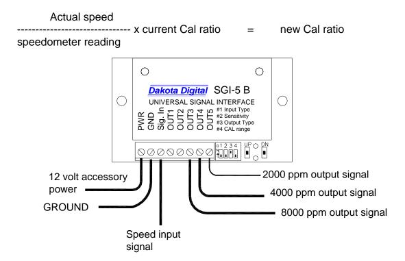
Convert an 8000ppm signal from an aftermarket signal generator to a 4000ppm or 2000ppm to run an OEM cruise control or fuel injection computer.
