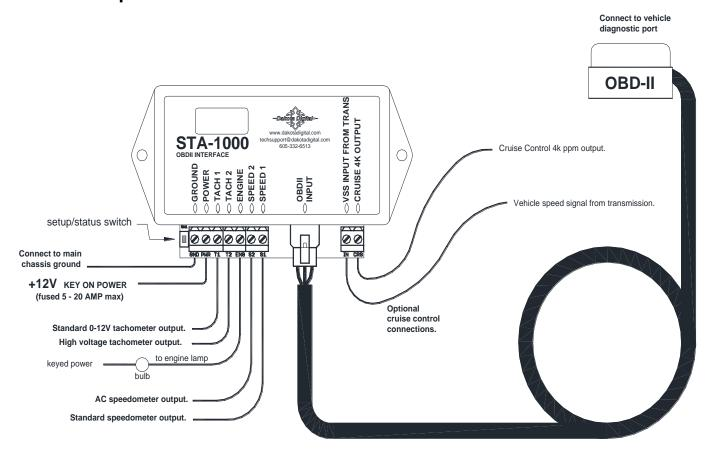
This unit has an input to read engine information from vehicles using the GM 1996-up OBD-II protocol, Ford 1996-up OBD-II protocol, some Chrysler 2000-up OBD-II protocol, or SAE CAN OBD-II protocol. CAN OBD-II is used on all vehicles 2008 and newer and some vehicles from 2004 – 2008. It provides speedometer, tachometer, and engine indicator outputs. Do not mount this in the module in the engine compartment; it should be mounted in interior of the vehicle.
