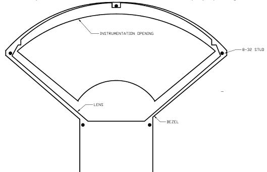
Next, take the supplied lens, with the lettering facing the front of the dash and place it in the chrome bezel. Lay a bead of RTV around the back side of the lens to secure it in place. After the RTV has cured, the display panel is ready to be placed on the bezel. If studs were supplied with the panel, screw them into the bezel and place a nut on them before placing the display system on it.
