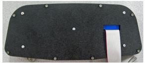
5. Using the screws that held on the original back plate and gauges, attach the new Dakota Digital gauge assembly to the bezel.
