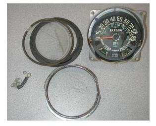
ng ear cutouts on the bezel or align the slot in the top of the lens to the mark made on the bezel earlier to ensure level installation of the lens. Remove the cardboard and/or plastic light tubes. Remove the rivets holding in the blue light covers. Cut a slot in the rear of the can for the ribbon cable to pass through.
