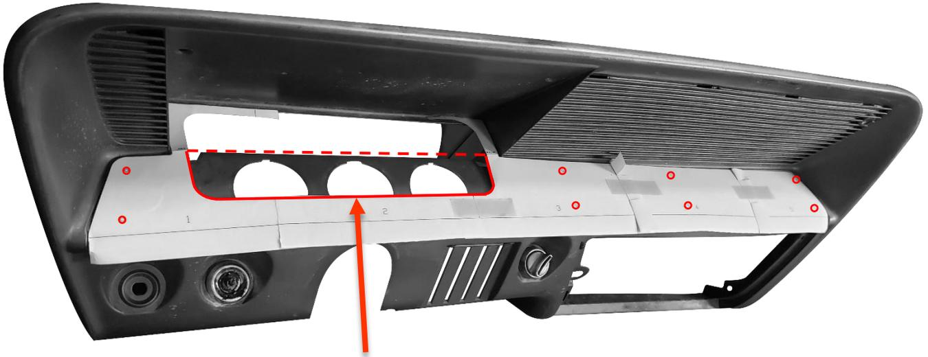
9. Carefully cut out traced section of dash and drill previously marked holes as needed with a size #27 drill bit. If adding an aftermarket radio, cut out the right side as well.
