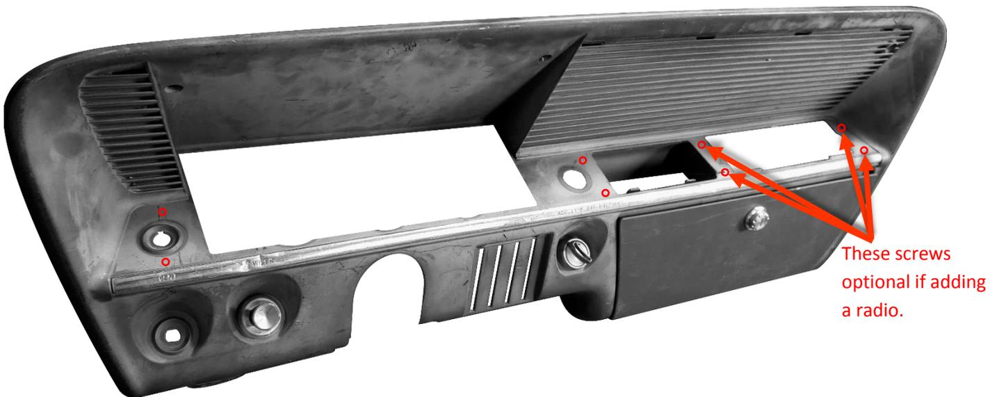
10. Remove protective film from lens. Assemble the VFD system by attaching the ABS backing panel and lens to the aluminum bezel using the six provided 3/4" standoffs and six of the 14 screws.
