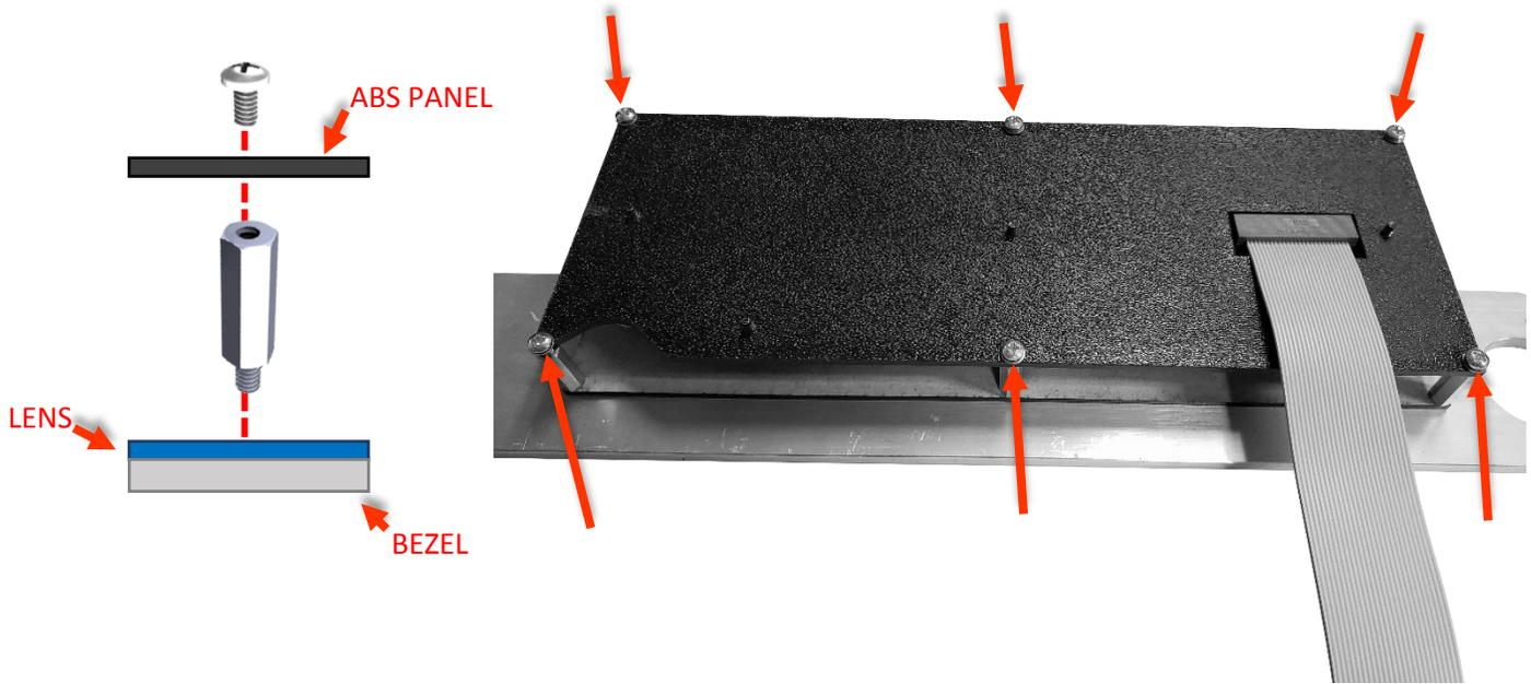
11. Insert the VFD system into the now cut-out dash opening. Secure using the remaining eight screws provided. If a radio will be installed, do so at this time. With a radio installed, you may use only four screws to secure the lens side of the system.
