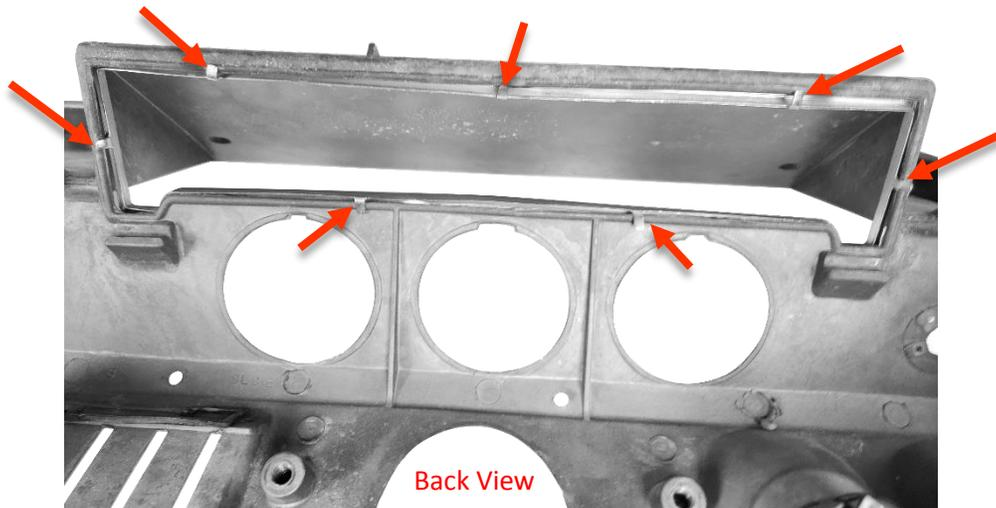
6. Place template on dash. Set the VFD system bezel on top of the template for alignment and secure template to dash using tape.
