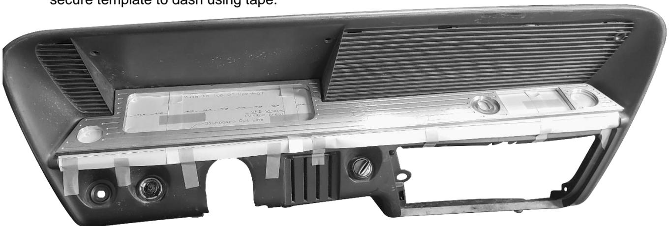
8. Cut out the line marked "Dashboard Cut Line" for a traceable outline of the dash area that needs to be removed. Trace this outline and mark screw holes. Cut out and trace other areas of the template to be removed as necessary.
