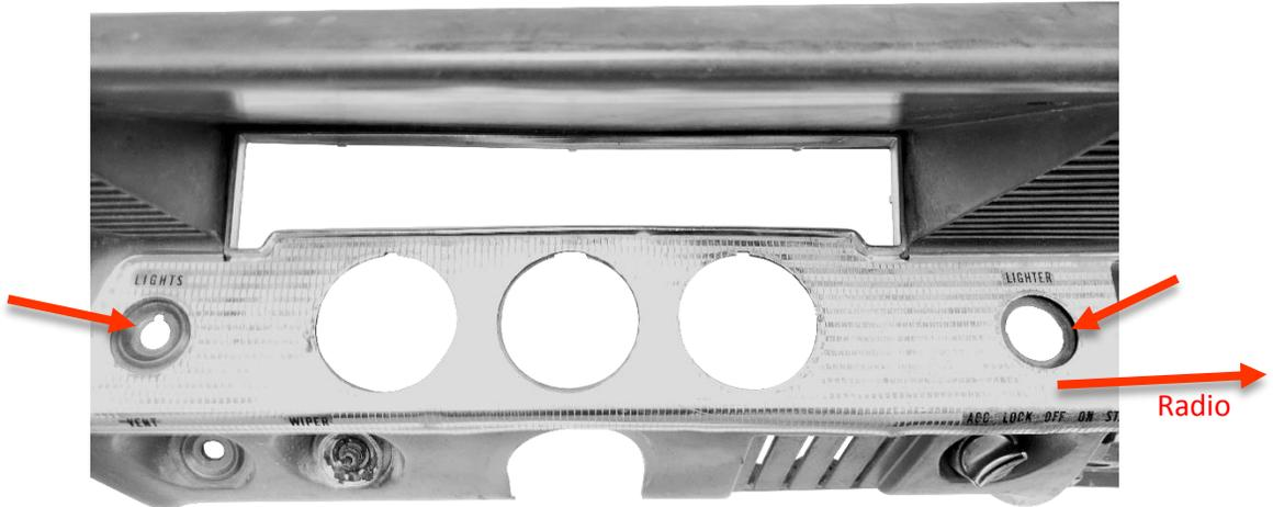
3. Straighten tabs holding on the stamped metal dash trim, and remove trim from the dash.
