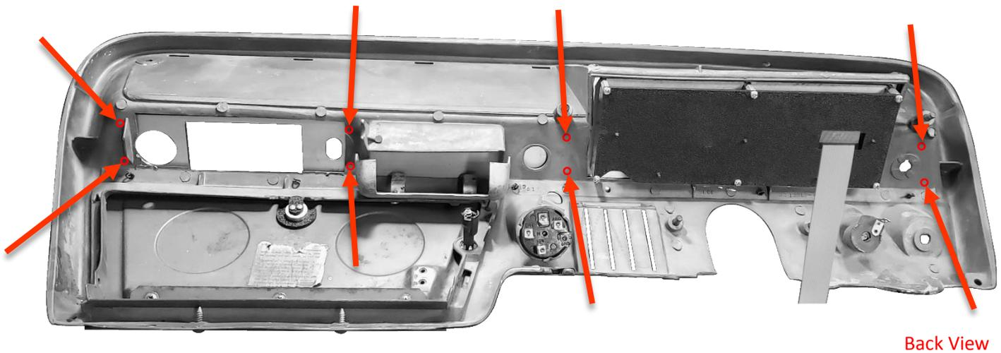
12. Reinstall stock headlight switch and cigarette lighter / ashtray. Refer to the VFD Main Manual for control box wiring and setup instructions to complete the installation.
