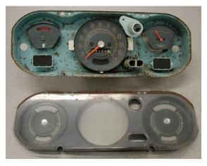
1. Remove the cluster from the vehicle. Remove the factory light bulbs and wiring from the back of the cluster. Remove clear lens and front gauge separator panel. The panels covering the outer two openings can be removed by bending open one of the retaining tabs. The plastic light guides can also be removed from the factory gauge can.
