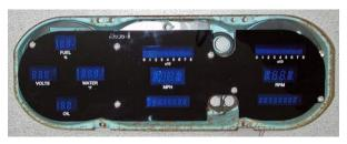
7. Use the two screws and black plastic washer included to hold it into the factory housing.
