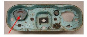
3. Remove the screw from the front of the battery indicator light on the top left as indicated by the arrow in the photo at left.
