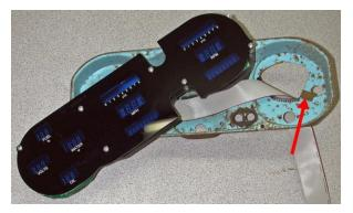
5. The metal tab, as indicated with the red arrow, needs to be bent as shown in the photo at right.
