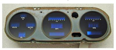
8. Replace the front gauge separator panel and clear lens. Block off pieces are included to be siliconed into the factory indicator holes in the bezel. Reinstall the gauge cluster onto the original bezel.
