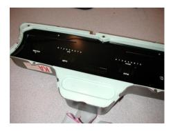
• Reinstall lower cover plate and rebend can lip to retain.
