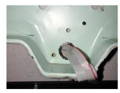
Install main display cluster in speedometer housing, pass ribbon cables through speedometer cable hole. Use supplied Phillips head screws to retain gauges. (Highlighted in photo)
