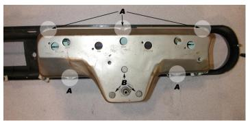
Remove stock gauges (Screws marked A in photo) and round clear lenses from bezel.
