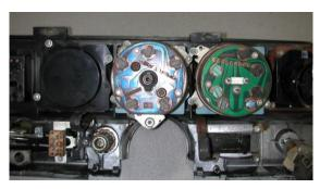
Install included #8-32 X  $\frac{1}{2}$ " hex standoffs on original gauge mounting studs, hand tightening as far as possible. Up to  $\frac{1}{16}$ " gap between standoff and hex of the original stud is acceptable. Be careful not to over tighten causing damage to the plastic risers.
