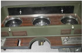
Remove the original gauges and set aside
