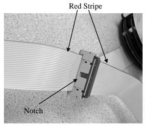
4. Install the gauges into the dash and connect the ribbon cables together. There is a notch on the blue cable end that corresponds with a slot in the inline connector.
