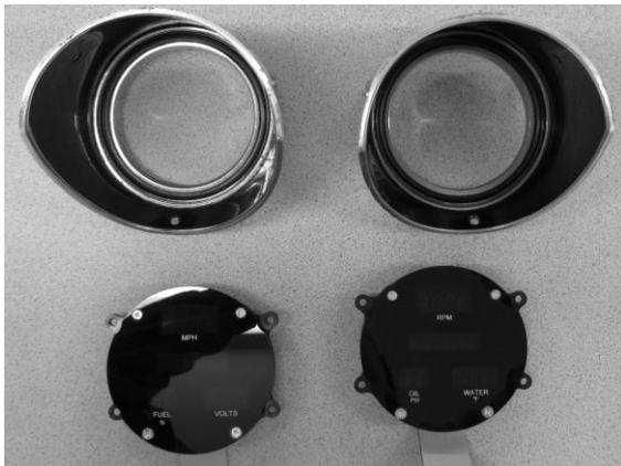
2. The speedometer gauge cluster will go onto the original speedometer bezel and the tachometer gauge cluster will go onto the original fuel gauge bezel.
