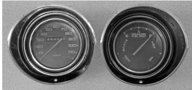
1. Remove the cluster from the vehicle. Remove the factory gauge cans from the original bezels. Keep the original screws as they will be reused.
