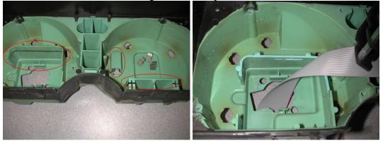
• Remove approximately 1/2" from the top part of the plastic divider on the speedometer side. Pass ribbon cable through center hole.
