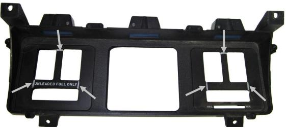
4. Spread a thin film of RTV silicone (not supplied) over the dashed line areas to hold the lens in place.
