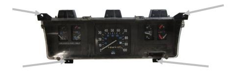
2. Remove the clear lens on the front as well as the circuitry panel on the rear. Retain all hardware for reassembly.
