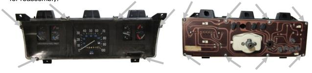
3. Now that the plastic housing is bare, make the six minor cuts as indicated in the following picture so the VFD3 displays will not be obstructed.
