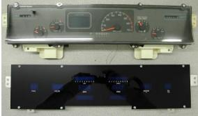
After removing the stock cluster from the vehicle remove the clear lens and black angled adapter plate.
