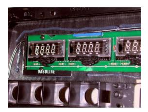
Put a bead of silicone around the gauge area being careful not to use too much or get too close to the edges where it may seep out into a visible area. Press lens into place.
