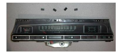
Remove Instrument cluster from vehicle. Remove four covers to expose screws in the indicator light area. Use a small screwdriver or pick from the rear of the cluster. Remove screws.
