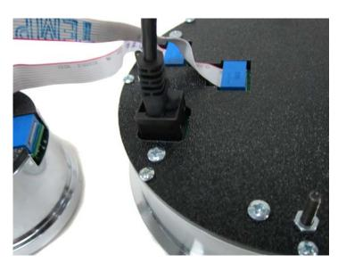
5. Connect the CAT5 cable to the backside of the large gauge and take care when routing this cable to the control box mounting location.
