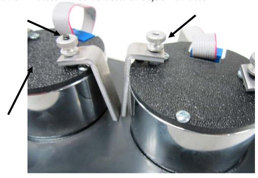
4. Be sure to make the connections correctly between the labeled ribbon cables from the main gauge to the lead from each small gauge.
