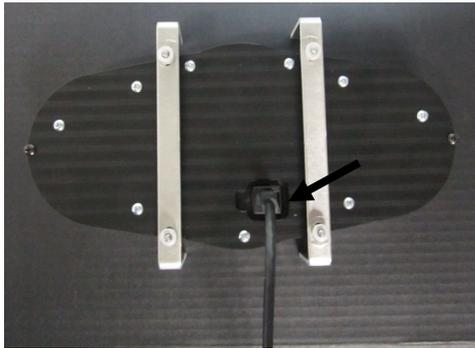
3. Attach the provided CAT5 Cable to the back of the VHX display and carefully route the other end to the control box mounting location and refer to the main manual for wiring instructions.
