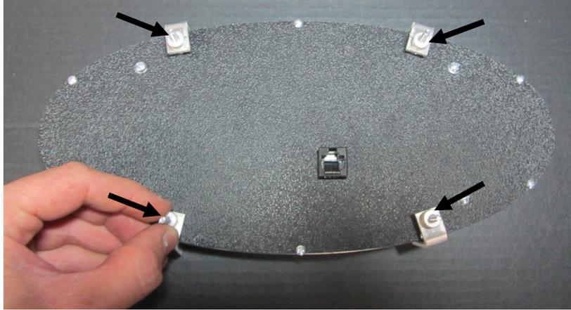
3. Remove the protective film, then, attach the provided CAT5 cable to the back of the VHX display. Carefully route the other end to the control box mounting location and refer to the main manual for wiring instructions.
