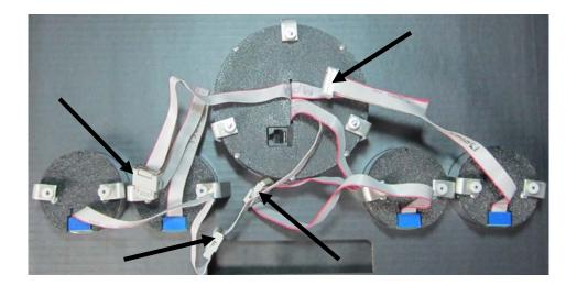
4. Connect the CAT5 cable to the backside of the large gauge and take care when routing this cable to the control box mounting location.
