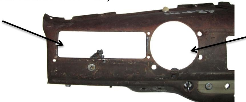
2. Place the VHX Speed/Tach gauge into place from behind, use the supplied flat head screws and the flanged nuts to mount the left two tabs to the dash; use stock hardware to mount the right two tabs.
