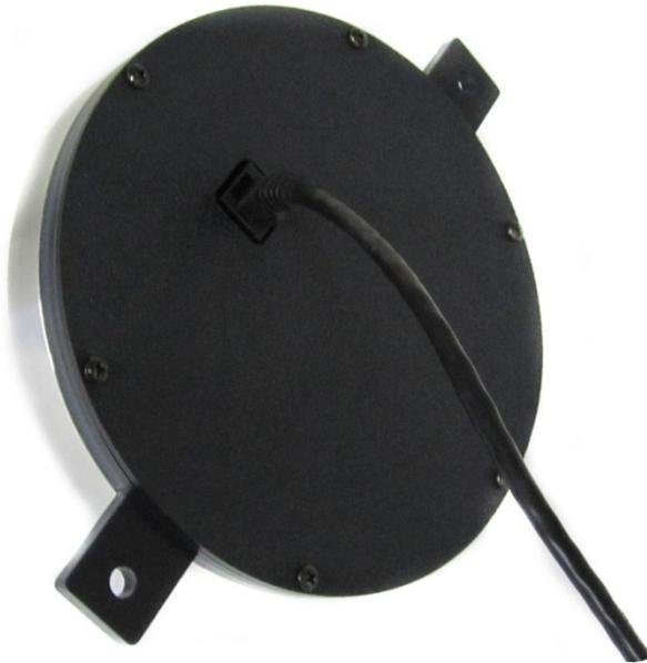
3. Connect the CAT5 cable to the system as the VHX cluster is installed into the dash. Watch carefully so you don't scratch or damage the lens or bezel, and take care when routing the CAT5 cable to the control box location.
