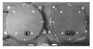
3. Connect the two halves of the new VHX system with the supplied 12" CAT5 cable. Also, route the 3' cable towards the control box location and connect it to the display.
