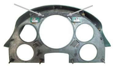
3. From the front, place the main gauge and the four small gauges through the bezel in the stock locations or arrangement of your choice; secure the gauges to the bezel by using the provided L-Brackets and thumb nuts. NOTE: the four (4) longer L-Brackets are used for the large main gauge.
