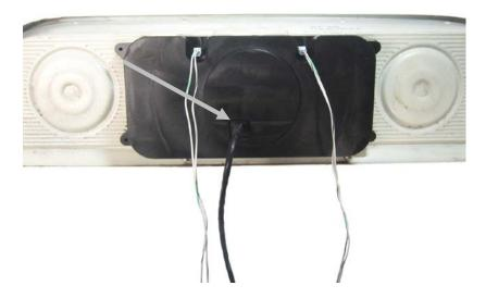
5. The gauge panel is now ready to re-install into the vehicle using stock hardware; take care when routing the CAT5 cable to the control box mounting location. Refer to the main manual to complete the VHX installation.
