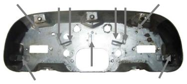
3b. To ease installation of the VHX System into the factory housing; drill out the indicated holes using a 3/16" drill bit. Before installation it is recommended to refinish the housing to prevent bare metal areas from rusting.
