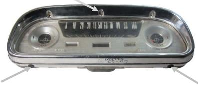
3a. The inside of the gauge housing will need to have the lens, gauges, and all the clips removed (front and back) so it is a bare panel only. ALL INTERNAL GAUGE MOUNTING AND SUPPORT TABS WILL NEED TO BE COMPLETELY REMOVED FROM THE HOUSING AND GROUND FLUSH TO ENSURE PROPER FITMENT. NOTE: DO NOT CUT THE BOTTOM DASH MOUNTING TABS ON THE REAR OF THE HOUSING.
