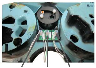
Right Blinker High Beam Left Blinker
