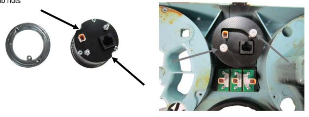
8. Remove the lens from the two large bezels and reuse the same screws to mount the bezels to the VHX speed and tach displays.
