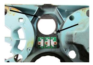
7. Remove the two screws that mount the bezel to the original clock; use the same two screws to mount the bezel to the VHX clock. From the front side of the housing, place the VHX clock into the clock opening, center the gauge, and secure the it using the clock mounting cup and the supplied thumb nuts
