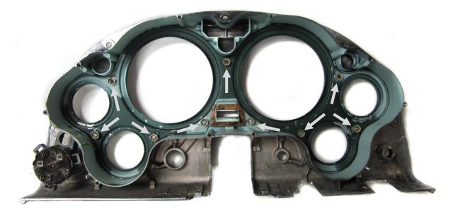
3. With the lenses and lens separator removed, place the included hole block off parts in the appropriate spaces (black arrows). We recommend using RTV silicone to secure the block off pieces in place. NOTE: Make sure the smooth side of the plastic with the part number is facing you when installing.
