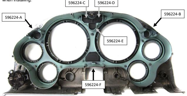
4. Using the 10 factory screws from Step One, secure the Dakota Digital gauge assembly to the bezel.
