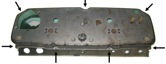
2. Remove the stock gauges, separator plate, and lens from the bezel. The only item to be reused is the original front bezel; the other pieces can be discarded. Now is a good time to clean the bezel and remove any dirt or old lens gasket material.
