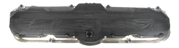
4. Secure the VHX system to the bezel using the eight (8) provided 6-20 x 1/2" screws.
