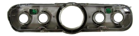
3. Remove the protective tape from the clear lens and insert the VHX system into the bezel. Watch carefully as you insert the system to avoid scratches or damage to the lens.
