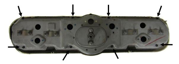
2. Remove the stock gauges and lens from the bezel. The bezel will be the only piece needed; all other parts can be set aside. Now is a good time to clean the bezel, or upgrade to a new one if desired.
