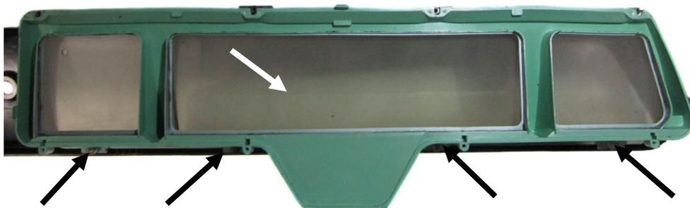
4. Mount the VHX system to the back of the bezel spacer using the stock hardware similarly to how the stock gauges were mounted. Note the longer screws are used for the top portion.
