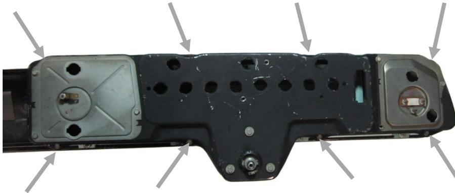
3. The stock clear lens is not needed but can be left in place if desired. To remove the clear lens, loosen the bottom four (4) studs and the lens will slip out. Make sure to re-tighten the studs after removing the lens
