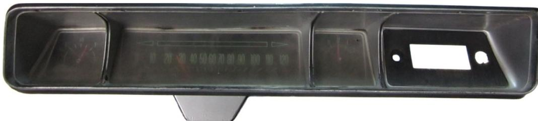
2. Remove the eight (8) screws that mount the stock gauges to the bezel. Retain the stock hardware for reassembly. The stock gauges can be set aside; they will not be reused.
