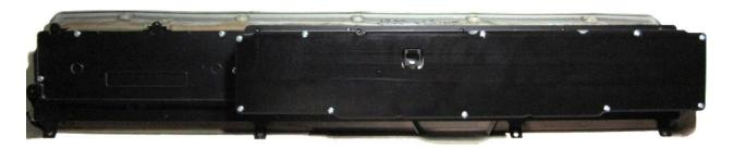
On 1967 models with a back lit heater control, you will have to modify the light housing to fit. Perform two cuts shown below and use the provided 10-32 X ¼" screw for the center mounting to the VHX bezel.
