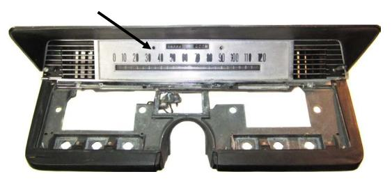
5. Remove the speedometer assembly so you are left with a bare gauge housing. The blue bulb shields can be left in place or removed if desired.
