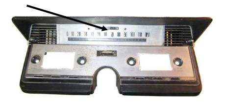
2. Remove the lower panel on the gauge bezel. Retain all hardware for reassembly.
