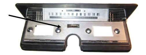
3. Remove the odometer assembly.
