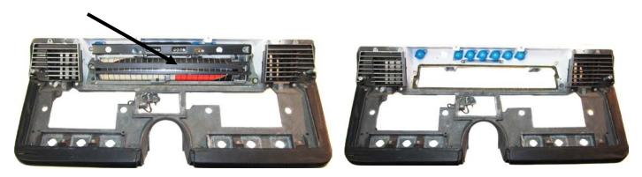
6. Separate the speedometer face from the gauge trim.
