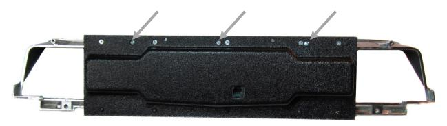
8. Attach the assembled gauge trim to gauge housing using five (5) 6-20 X 5/8" screws.
